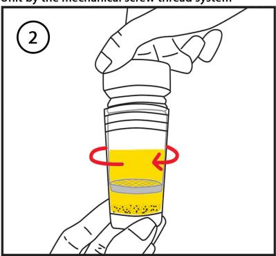
Unfasten the Filter Unit (counter-clockwise) from Container Unit. Use the concentrated urine sediment volume left in the Container Unit for analysis
